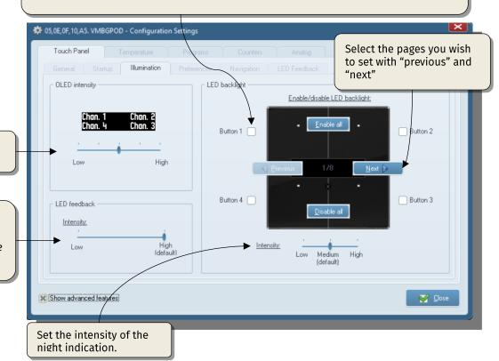
Set the intensity of the OLED display (during operation)
