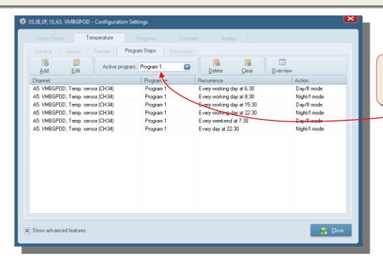
**Do not forget to select the active program!** This is only possible if Velbuslink is connected.
